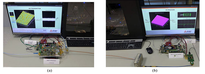
Fig. 22. (a) “CPHY in T2” transmitter: The DVB-T2 modulator (front) and the CPHY Tx interface board (rear), the CPHY transmitter control display. (b) “CPHY in T2” receiver: The DVB-T2 frame splitter (front), the CPHY Rx interface board (rear), the CPHY receiver control display.
