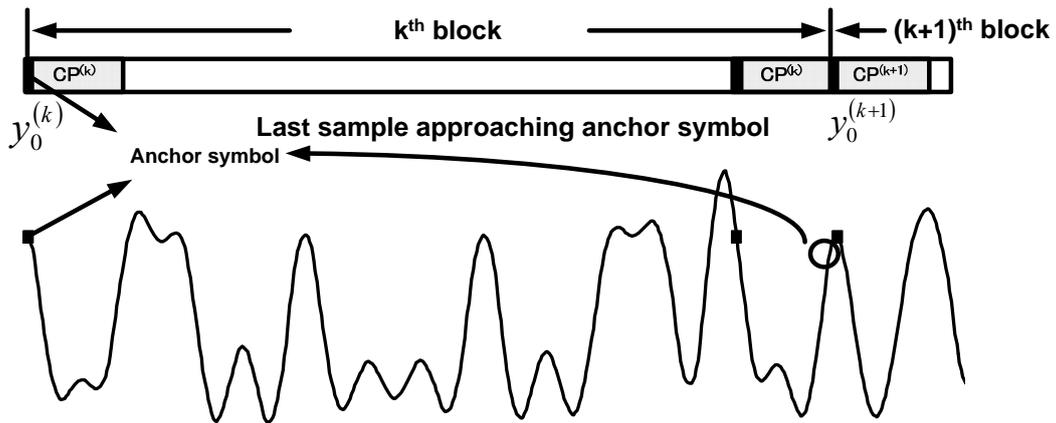
Fig. 2 Anchor symbol and phase continuity
