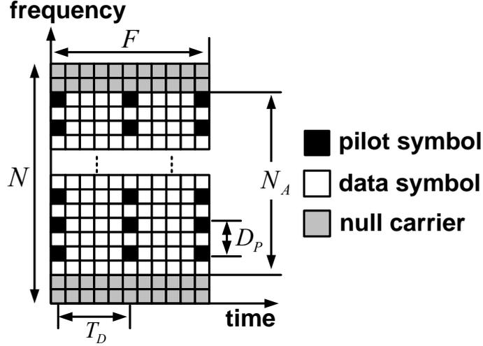
Fig. 4 Proposed frame format using SC-OFDM data blocks and hybrid SC-OFDM blocks
