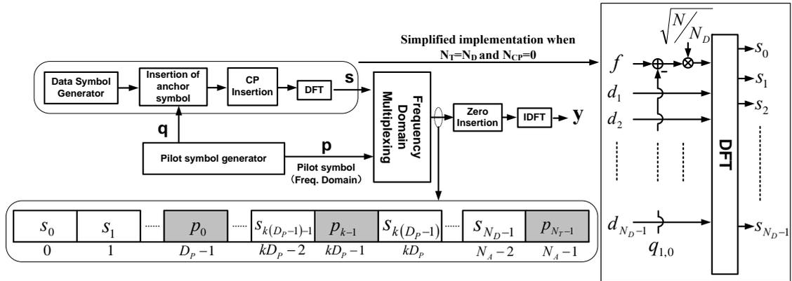
Fig. 5 Proposed hybrid SC-OFDM transmission scheme when  $N_{CP} = 0$
