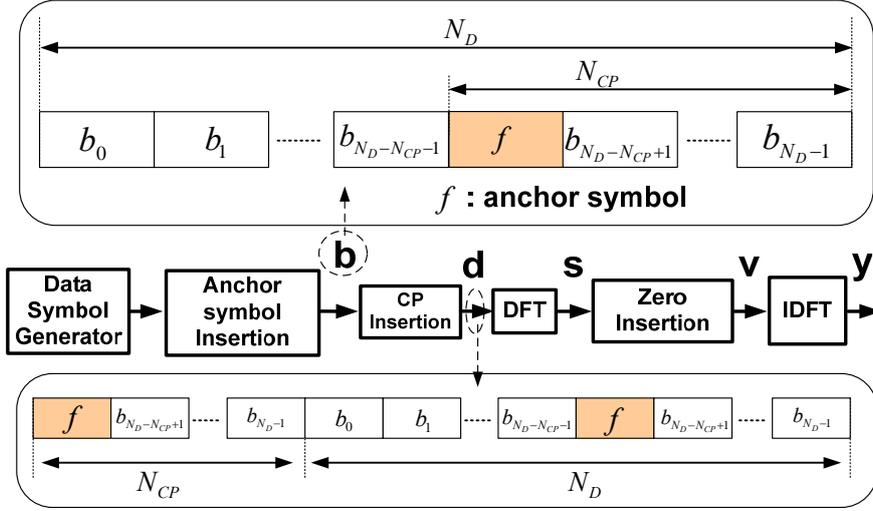
Fig. 1 Proposed SC-OFDM transmission scheme
