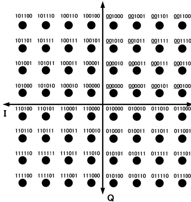
Fig. 3 An example of mapping for the anchor symbol using 64QAM by fixing two MSB in the upper right hand quadrant: fixed bits are underlined in the figure
