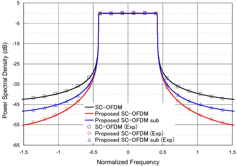
Fig. 6 Power spectrum performance of the proposed schemes for 64QAM
