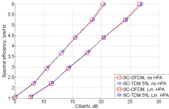
c) 4-channel usage: outer channels with optimized parameters
