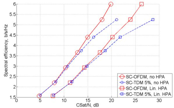
f) 4-channel usage: inner channels, parameters optimized for outer channels
