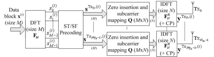
Fig. 1. SC-FDMA transmitter with ST/SF precoding ( $M$  out of  $N$  allocated subcarriers,  $N_{\text{Tx}}$  transmit antennas).
