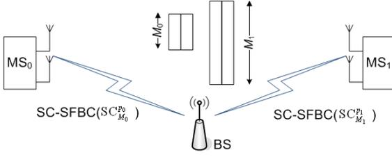
Fig. 3. MU-MIMO SC-SFBC: two users with spectral overlapping.
