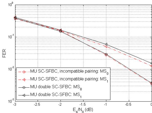
Fig. 9. Performance comparison of SC-SFBC with incompatible subcarrier pairing and MU double SC-SFBC with reduced decoding complexity, an example for  $M_0=60$ ,  $M_1=20$ , QPSK 1/2,  $N_{Rx}=4$ .
