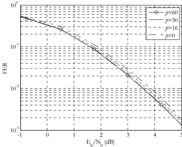
Fig. 8. 2x2 SC-SFBC with variable  $p$ : 3kmph, 120 localized subcarriers, QPSK 1/2, MMSE decoding with ideal channel estimation.
