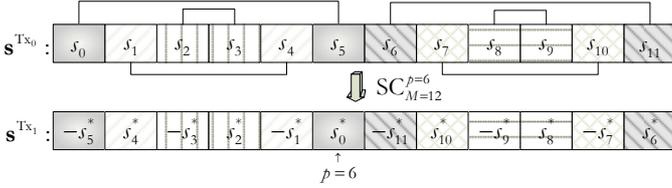
Fig. 2. SC-SFBC precoding; example for  $M=12$ ,  $p=6$ .
