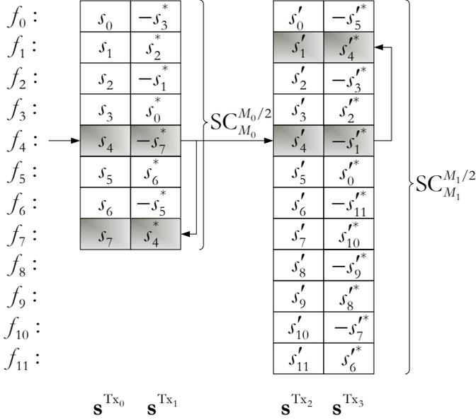
Fig. 4. MU Double SC-SFBC with incompatible pairing of subcarriers; example for  $M_0=8, p_0=4, M_1=12, p_1=6$ .
