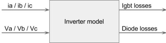
Figure 6. Inputs and outputs of the inverter model
