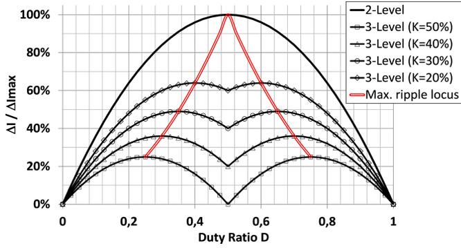
Fig. 7. Comparison of ripple functions between two-level and three-level boost converters for different  $K$  factors.
