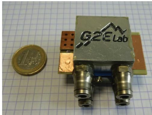
Fig. 12: 3D module with water cooling system
