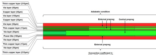
Fig. 20: PCOC module geometry for thermal simulation
