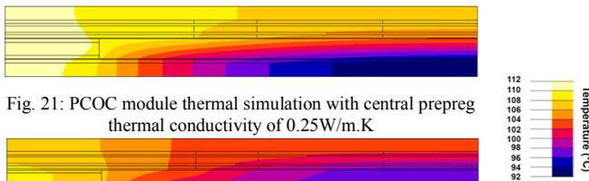
Fig. 21: PCOC module thermal simulation with central prepreg thermal conductivity of 0.25W/m.K
