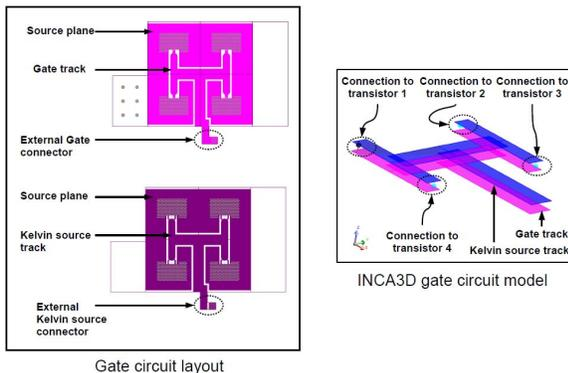
Fig. 13: Gate circuit layout and associated INCA3D model
