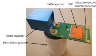
Fig. 2: PCOC module with DBC and PCB realization [6]
