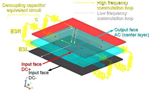
Fig. 9: PEEC simulation of PCOC module with four parallel commutation cells and decoupling capacitor on module edge
