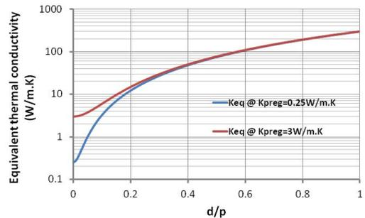
Fig. 19: equivalent thermal conductivity in function of  $d/p$  ratio
