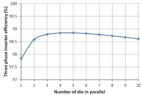
Fig. 6: Three phase inverter efficiency in function of number of die in parallel
