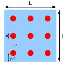
Fig. 18: Via region geometrical parameters definition
