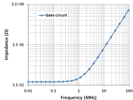
Fig. 16: Gate circuit impedance
