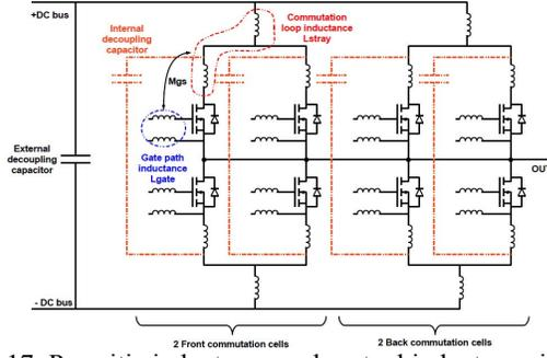
Fig. 17: Parasitic inductance and mutual inductance in the module
