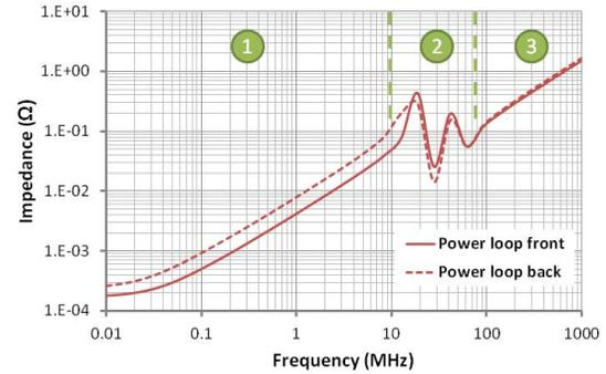
Fig. 10: front and back power loop impedance simulation with decoupling capacitor on module edge
