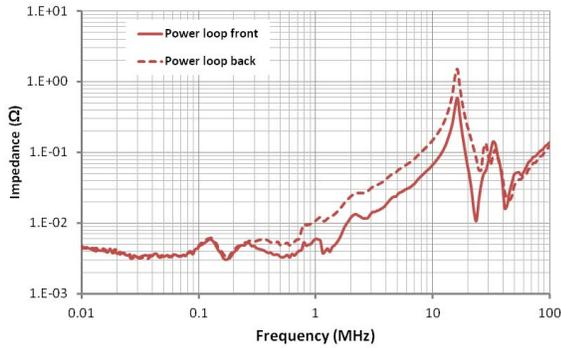
Fig. 12: Front and back loop impedance measurement on mock prototype
