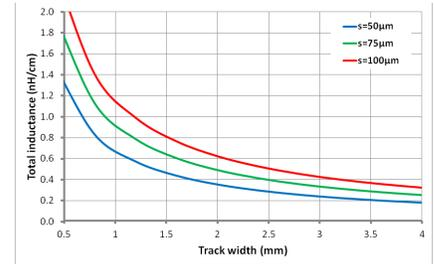
Fig. 15: Busbar inductance in function of track width and spacing
