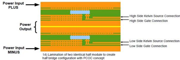
Fig. 3: PCOC module with embedded die overview
