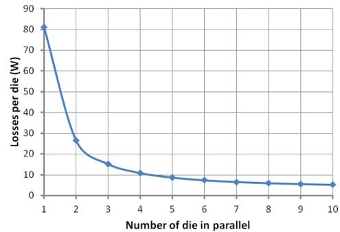
Fig. 7: Loss per die in function of number of die in parallel
