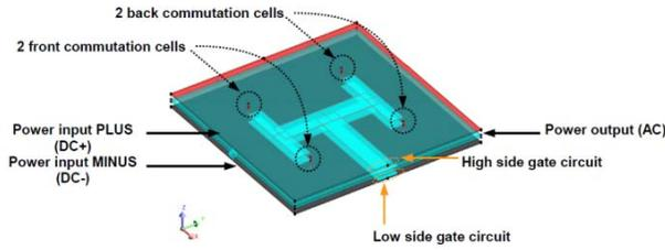
Fig. 8: PEEC simulation of PCOC module with four parallel commutation cells
