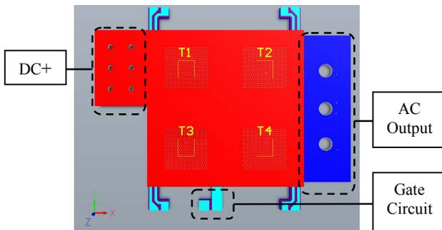
Fig. 4: High side sub-module prototype top view
