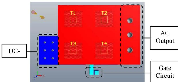
Fig. 5: Low side sub-module prototype top view
