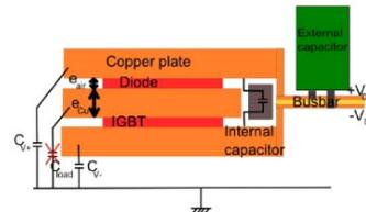
Fig. 1: The PCOC electrical concept; switching cell integrated in the busbar [5]
