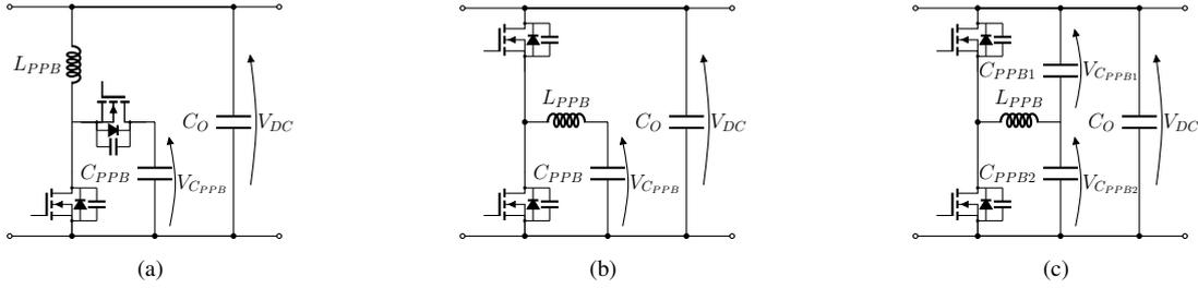
Fig. 2: Examples of different parallel Power Pulsating Buffers. a) Boost b) Buck c) Symmetrical Half Bridge (HB)
