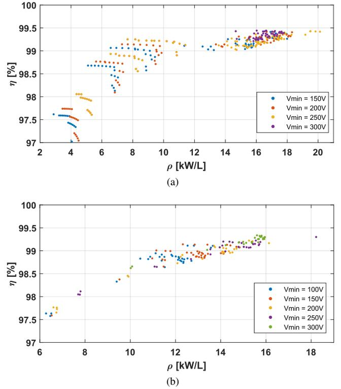
Fig. 8: Results of the optimisation presented in the Power Density vs. Efficiency domain. a) X6S capacitor/planar inductor with a thermal coefficient of 5 cm<sup>3</sup>/W for the cooling system. b) X6S capacitor/PCB-embedded inductor with thermal coefficient of 5 cm<sup>3</sup>/W.
