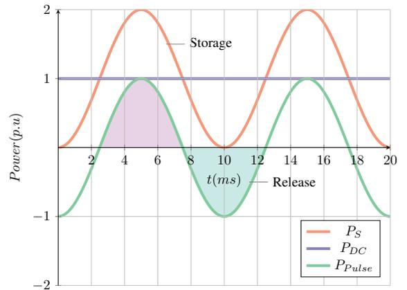
Fig. 1: Typical power waveforms for an AC/DC converter.  $P_S$  is the power on the AC side,  $P_{DC}$  is the power on the DC side and  $P_{Pulse}$  is the power that needs to be buffered by the PPB.
