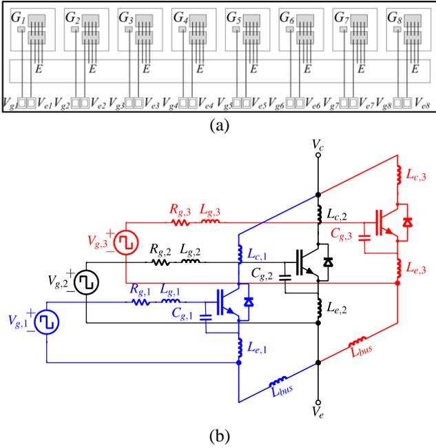
Fig. 5. Individual Gate drive of multi dies module (a) layout of the substrate and (b) Individual gate driven equivalent electrical schematic
