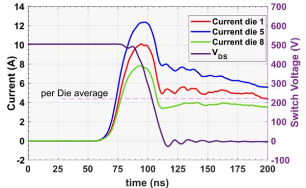
Fig. 17. Experimental waveforms of SiC prototype for a delay of  $\delta t = [0, 2.2, 0.8]\text{ns}$  for dies 1, 5 and 8 respectively.
