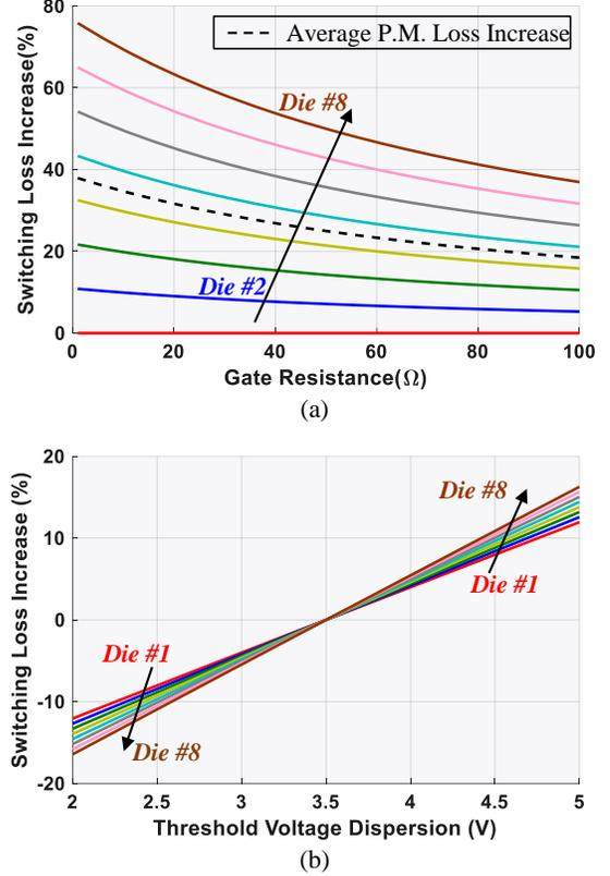
Fig. 4. Turn-on switching losses across 8 parallel dies (a) with increasing gate resistance, and (b) increasing threshold voltage dispersion
