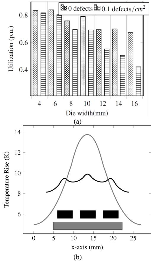
Fig. 2. Benefits using smaller dies (a) yield of a wafer as a function of die width (mm) for two defect densities, and (b) temperature rise across the linear distance of a single die (gray) against three dies with a similar total area (black)
