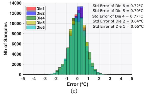
Fig. 10. Experimental junction temperature measurements from prototype of the Fig 19 (a) TSEP as per (5) in function of the temperature variation on the gate of a single IGBT die ( $R_{gint} = 13 \Omega$ ) under changing dc bus voltage and switching frequency; Temperature dispersion: (b) a power module with 13 $\Omega$  internal gate resistance; and (c) a power module with 2 $\Omega$  gate resistance
