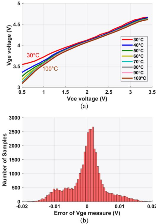
Fig. 12. Experimental on-state voltage measurements from prototype of the Fig. 19: (a) increasing blocking voltage of an inactive die with changing gate voltage and temperature; and (b) Distribution of the collector emitter voltage error samples using the described method with selective gate driving and the actual measurement
