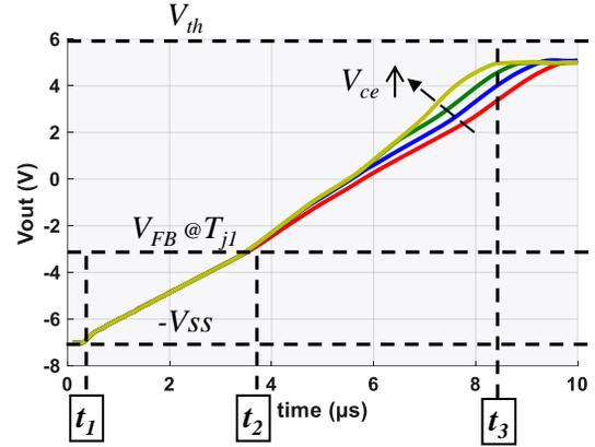
Fig. 8. Experimental waveform of the gate voltage of the inactive die with a constant injection current, and with various blocking voltages, from 0V to 3V, across the inactive die at 25°C (IGBT ref: CM150TX)
