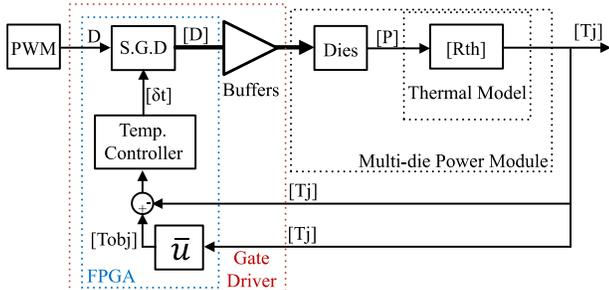
Fig. 18. Selective gate driving: reduction of peak junction temperatures with application of a driving profile for a power module with multi-gate (MG) access compared to the reference single gate (SG) power module
