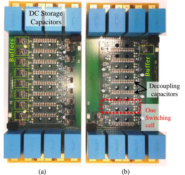
Fig. 15. Experimental prototype composed by 8 paralleled SiC MOSFETs (a) Selective gate driving module (b) Classical driving module
