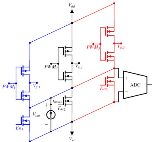
Fig. 7. DC gate injection circuit for a 3 die system with a measurement current  $I_{meas}$  and measured gate voltage corresponding to  $V_{out}$
