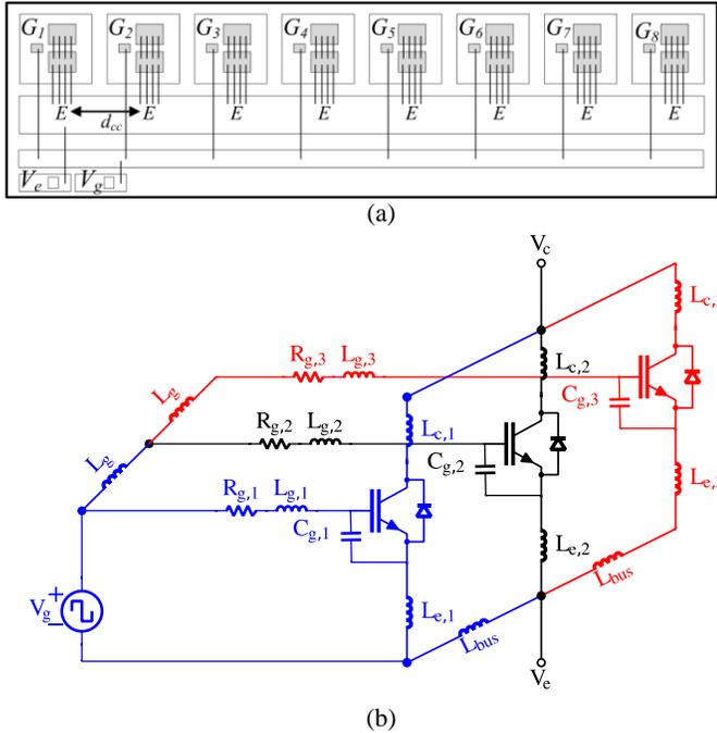
Fig. 3. Gate driving multi dies module (a) Substrate connection with a common emitter/source layout for 8 parallel dies (b) Electrical schematic of the parasitic network of three parallel dies in common emitter
