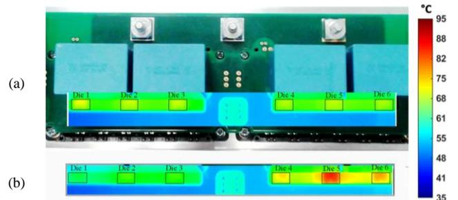
Fig. 13. Temperature distribution of the dies of the prototype of Fig.18 at 78A (a) Thermo-controlled (b) Classical gate driving
