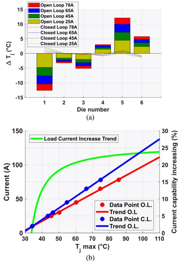
Fig. 20. Application of temperature balancing the prototype power module at 500V and 10 kHz (a) difference in temperature relative to the mean temperature with balanced and unbalanced temperatures and (b) load current handling capability increase
