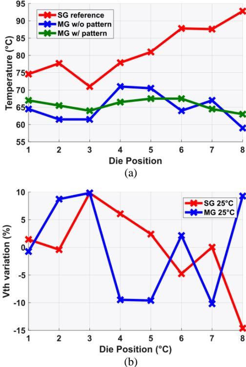
Fig. 16. Experimental data of the classical single gate (SG) and the Multi-gate access (MG) power modules (a) reduction of peak junction temperatures with and without Fixed Delay Stress Steering (w/o pattern) (b)  $V_{th}$  variation on the dies composing the modules
